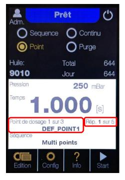
It is possible to start the program at a specific dosing point and/or repeat if required. Simply press the 2 red areas and select the desired dosing point and/or repeat.
