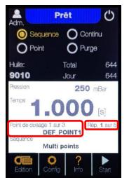
It is possible to start the program at a specific dosing point and/or repeat if required. Simply press the 2 red areas and select the desired dosing point and/or repeat.
